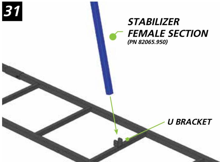
**1 3/4" BOLT, LOCK NUT - WRENCH TIGHTEN**
