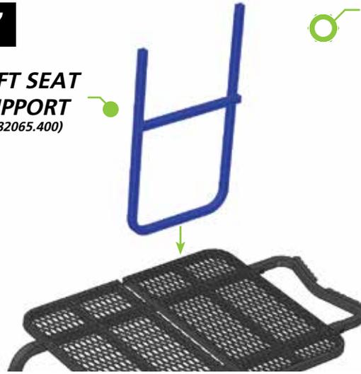
**2 1/2" BOLTS, LOCK NUTS - WRENCH TIGHTEN STEP 5**
