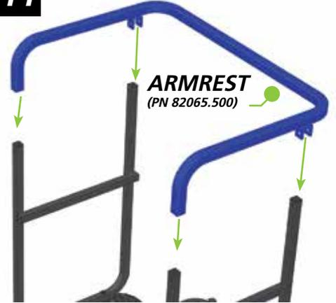
**1 3/4" BOLTS, LOCK NUTS - WRENCH TIGHTEN**
