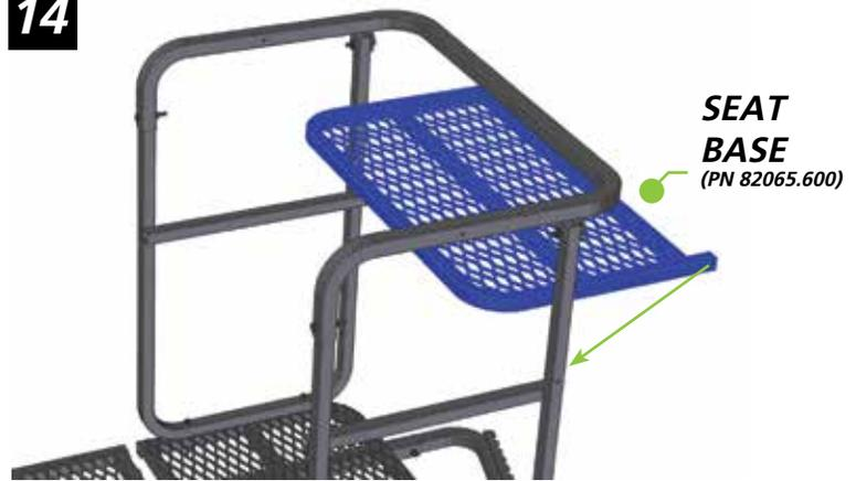
**2 1/2" BOLTS, LOCK NUTS - WRENCH TIGHTEN**
